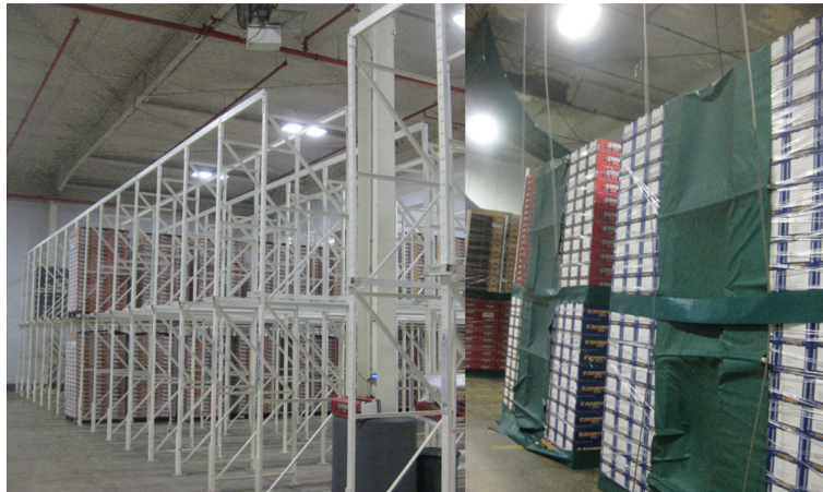
FIGURE 13.2 Commercial-scale treatment of peach and nectarine fruits after harvest at Summerripe, Fresno, California. Firm-ripe fruit are maintained at 20°C, 90–95% R.H. for 48 h (left), followed by forced-air cooling (right) prior to cold storage.
