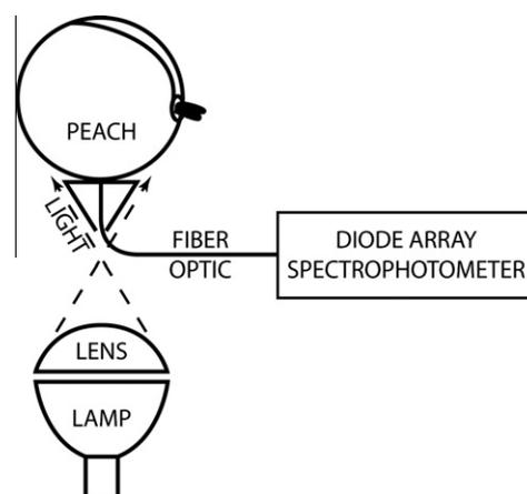
Fig. 1. Illustration of the setup used to nondestructively measure the interactance of intact peaches.
