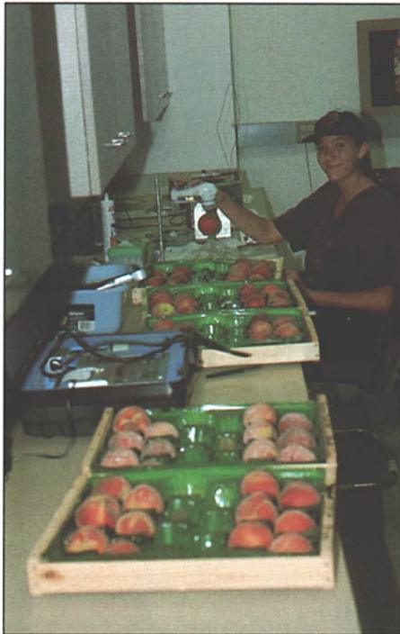
Some of the fruit were abraded to study the role of injury in inking. The fruit were abraded with a rotatable automatic toothbrush and a fruit holder.
